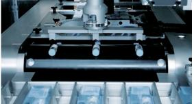
Compact rotating unit for turning the blisters through 180°
